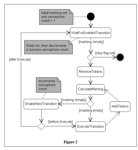
A new marking is calculated twice per loop, the first time after removing tokens from input places. This marking may be empty due to a conflict or because only one transition was enabled in the previous marking, but this does not produce deadlock. If the new marking calculated after removing tokens still has enabled transitions, the semaphore is released, enabling any waiting thread to process a remaining transition concurrently.
